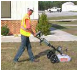
Ground Penetrating Radar
